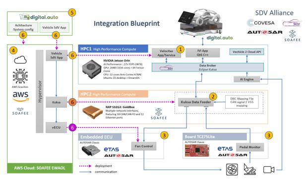
Figure 1: Integration Blueprint based on SDV Alliance standards and technologies.
